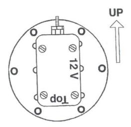
Due to variations in the inside flange diameter of some tanks, clearance or alignment problems may be encountered. It may be necessary to slightly grind or file the protruding area of the sending unit, or a portion of the tank flange. Ensure the gas tank, sending unit and dash gauge are securely grounded.
