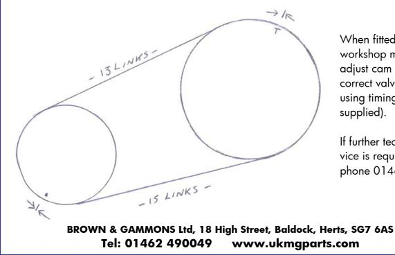
When fitted as original workshop manual, adjust cam timing to get correct valve opening using timing wheel (not supplied).
