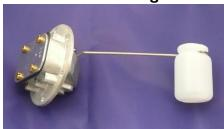
The Smith series petrol tank sending units are an antiquated design and require careful installation if leakage is to be avoided. Our reproduction units incorporate fuel resistant rubber gaskets and seals which will provide improved performance over the original cork gaskets, but they still require careful installation. The very nature of this design is such that the hollow rheostat cavity will fill with fuel. This does not pose a safety hazard as long as the cover plate is in place.
