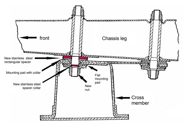
**Note:** The cross section shown is that of a chrome bumper car. A rubber bumper cross member is virtually identical apart from a fabricated metal spacer above the cross member and part of it.
