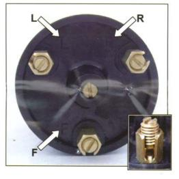
signalling a left turn. If the meter shows continuity, L means Left in your application. If there is no continuity, move the lead on the L terminal to the R terminal and move the lever to the left again. If there is continuity now, the L means right and R means left as far as the wiring is concerned.
