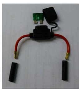
In standard form the MGB and BGT V8 overdrive switch wire is not run through a fuse. This can have dramatic results if a short occurs since the resultant fire can literally melt the rest of the harness. It's therefore a sound idea to fit a fuse using the kit as shown in the picture on the left.
