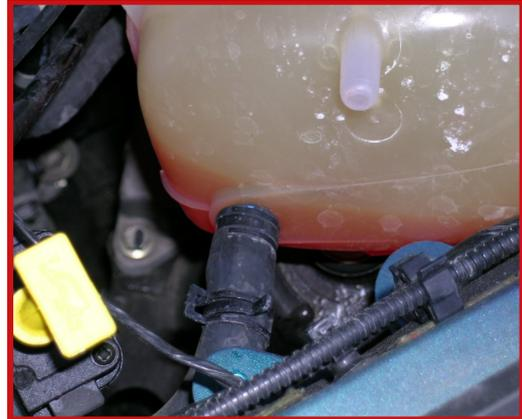
**4** Clip the sensor to the bottom of the new expansion tank and fit the two supplied metal tubes into the plastic tank pipes as this will help to prevent the pipes from crushing when tightening the hose clips. Then refit tank in reverse order. Then top up with fluid from the old tank. You may find it necessary to top up with new anti-freeze/ water mixture.
