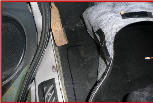
**11** Lift front section of carpet and run wire beneath carpet and up to centre console.
