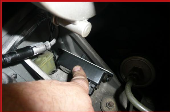
**5** Secure ECU to triangular reinforcement section on left hand side of boot, with the aid of fir tree clip and double sided tape.
