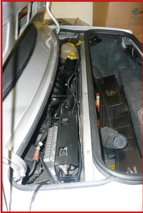
**7** Route expansion tank sensor wire behind engine ECU mount plate and over to tank on right-hand side of car. Connect to sensor beneath tank, and secure wire with tie wraps along rear panel.
