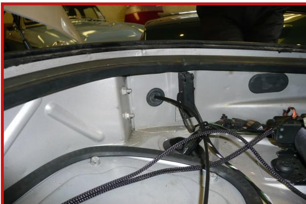
**9** Route long part of harness through grommet on left hand side just above car main harness grommet. You will need to make a hole in original grommet.
