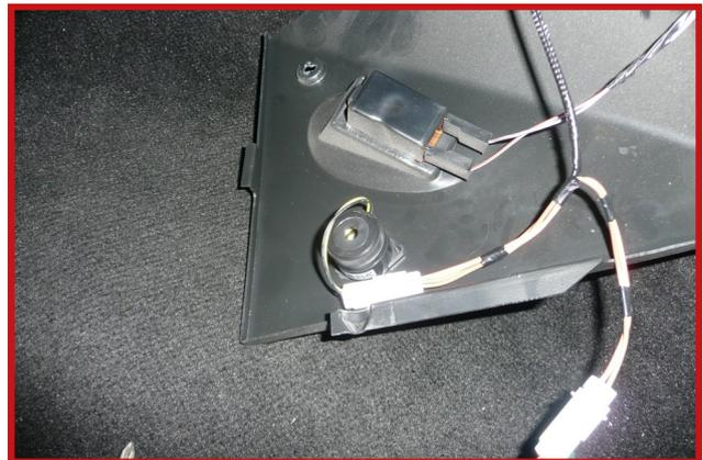
**13** Remove the left hand side panel to gain access to the rear of switches.
