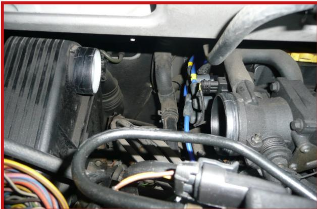
**2** Open boot, remove rear mesh cover, remove airfilter to throttle body link pipe
