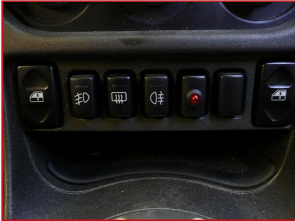
**14** Drill a 8mm hole in a spare switch blank. Alternatively, if you have an early car, drill a hole in the centre of the switch mount. Fit lamp and connect wires (see picture which shows how unit comes apart for fitting).
