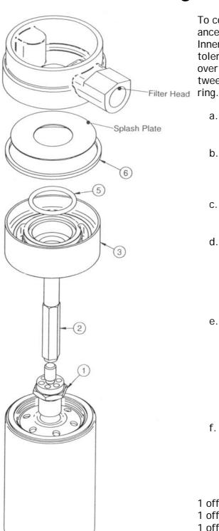
To compensate for the variations in Filter Head tolerances, the Spin On consists of three parts - Spin On Inner, Spin On Outer and an O ring. The variations in tolerances are taken up by the Spin On Outer sliding over the Spin On Inner. The integrity of the seal between the Inner and Outer is maintained by an O ring.
